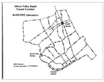
BART Burrow was proposed. Shown at <a href="http://www.electric-bikes.com/prt/bart-prt.html">http://www.electric-bikes.com/prt/bart-prt.html</a>, it outlined 91 miles of ATN guideway with 117 stations. That proposed network covers the Golden Triangle and downtown San Jose. Now, we can plan a network that matches our current needs.
