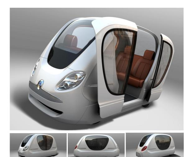
The exterior is compact with optimal interior space. Ease of access is provided by large, automatically operated, sliding doors. Although stations might be featured on both sides of the tack, the vehicle will only feature sliding doors on one side. Access to the vehicle will be ensured from the platform in adaptation of the platform design. The opening width of the doors allows for wheelchair or pram access from the platform which is flush with the vehicle floor.
