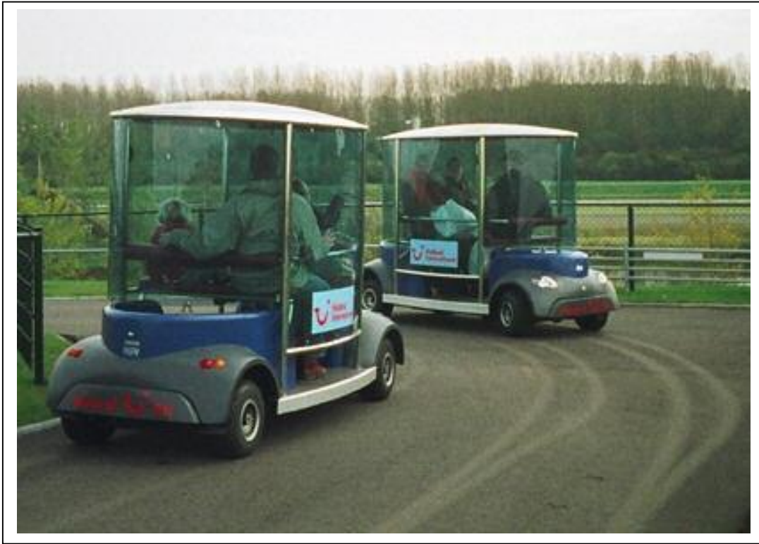
FIGURE 1 The 2getthere system. Note how the wheel tracks of numerous T-Pods verify the accuracy with which the guideway (defined by magnets under the surface) is followed.
