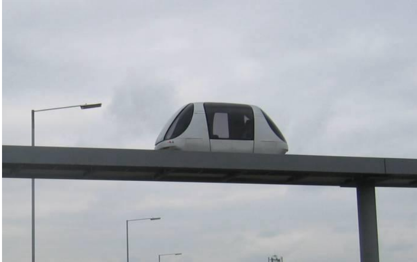
Figure 3 ULTra Vehicle on Elevated Track
