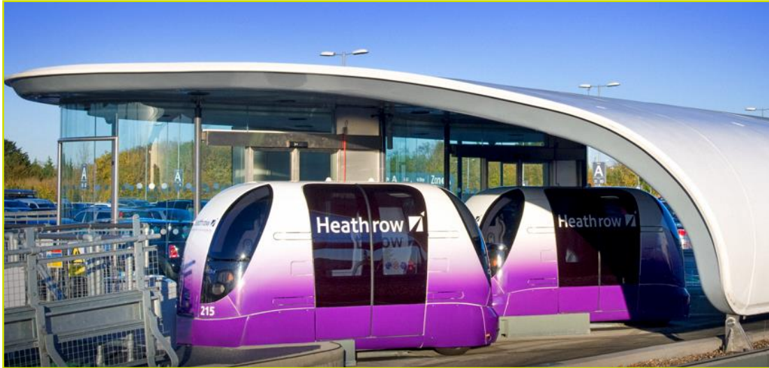
Figure 3 “Heathrow pod” PRT system
