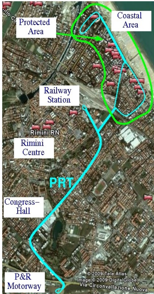
Fig.1: Schematic outline of the analyzed PRT network at Rimini, Italy with major activity centers along the PRT line. The thick cyan lines are bidirectional PRT lines while thin lines are unidirectional.
