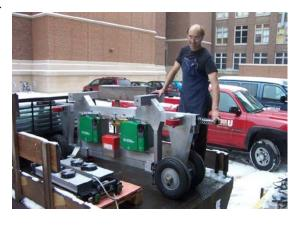
throughput is much greater. LIMs can be used only on a special running surface – a guideway, usually elevated to avoid congestion. The picture shows the vertical chassis I designed and its builder, Robin Russell. A pair of LIMs built by Force Engineering, Ltd, lie on the lower left in the picture, not yet installed. ITNS is designed in such a way that no connection with the Internet is needed. We are hack proof!
